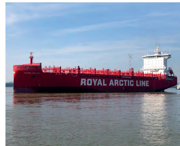
Picture: TUKUMA ARTICA, Container carrier, ice class +1A Polar code, 2,150 teu. Built and delivered in January 2020 by Chinese shipbuilder GWS to Royal Arctic Line. Designed by Deltamarin. Photo: Royal Arctic Line.
