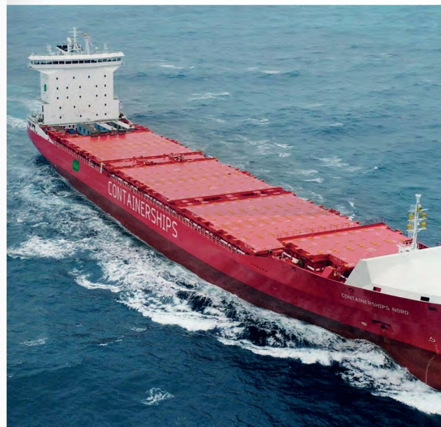
Picture: **CONTAINERSHIPS NORD**. Container carrier, Ice class 1A, 1,400 teu, built by Chinese shipbuilder GWS and delivered on 12 December 2018. This is the first LNG-powered vessel delivered to CMA CGM through its subsidiary Containerships.
