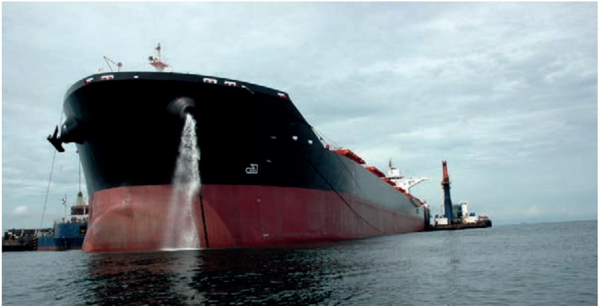
IMO's ballast water convention requires vessels to exchange ballast water at sea, which can result in high stress on the hull, especially if procedures are not correctly followed.
